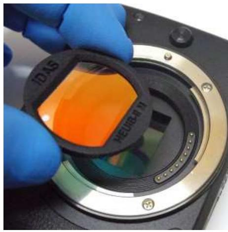
2) Align the aperture of the M filter with the rectangular aperture of the body mount. You can rotate the M filter even after the insertion.
