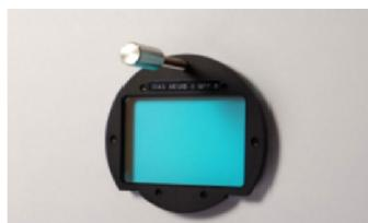
1. Softly screw in the bundled hand screw into the R filter.
