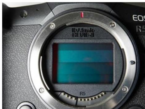
First, hold the R5 Filter so the crescent part of the R5 mates with the dented portion of the body mount. Then, slowly mate the rest part of the R5 with the dented portion.
