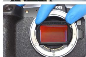
2. Softly insert the RP Filter into the dented portion of the body mount.
