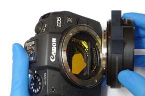
4. Mount a lens or mount adapter while holding the camera body so the body mount become upwards.
